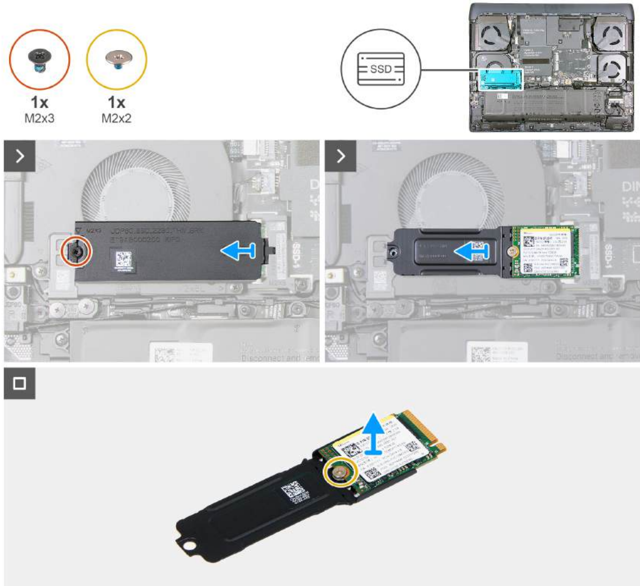
Figure 23. Removing the M.2 2230 SSD in slot 1
