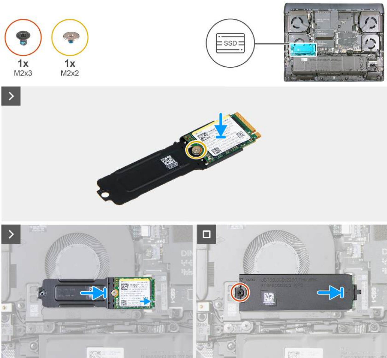
Figure 24. Installing the M.2 2230 SSD in slot 1
