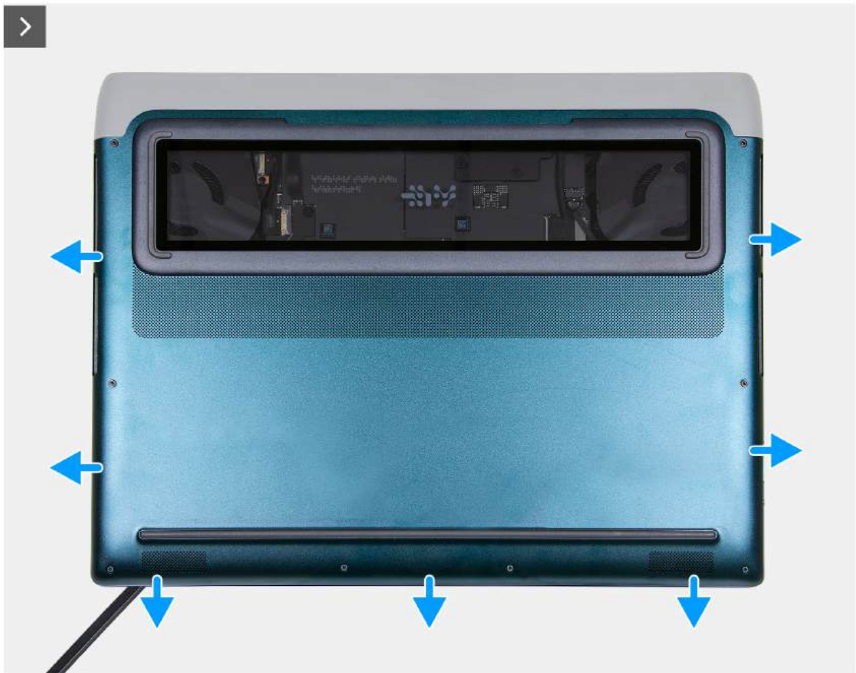
Figure 10. Prying the base cover
