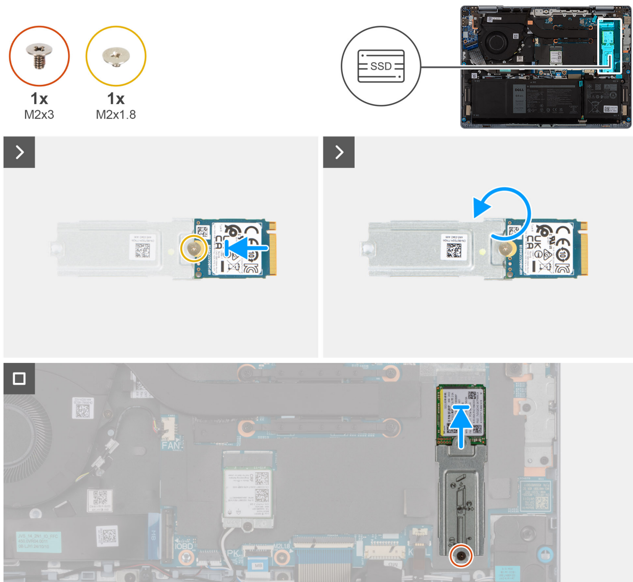
Figure 23. Installing the solid-state drive
