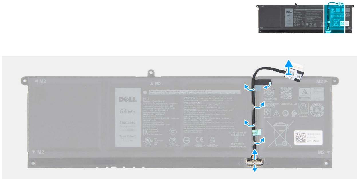
Figure 20. Disconnecting the battery cable
