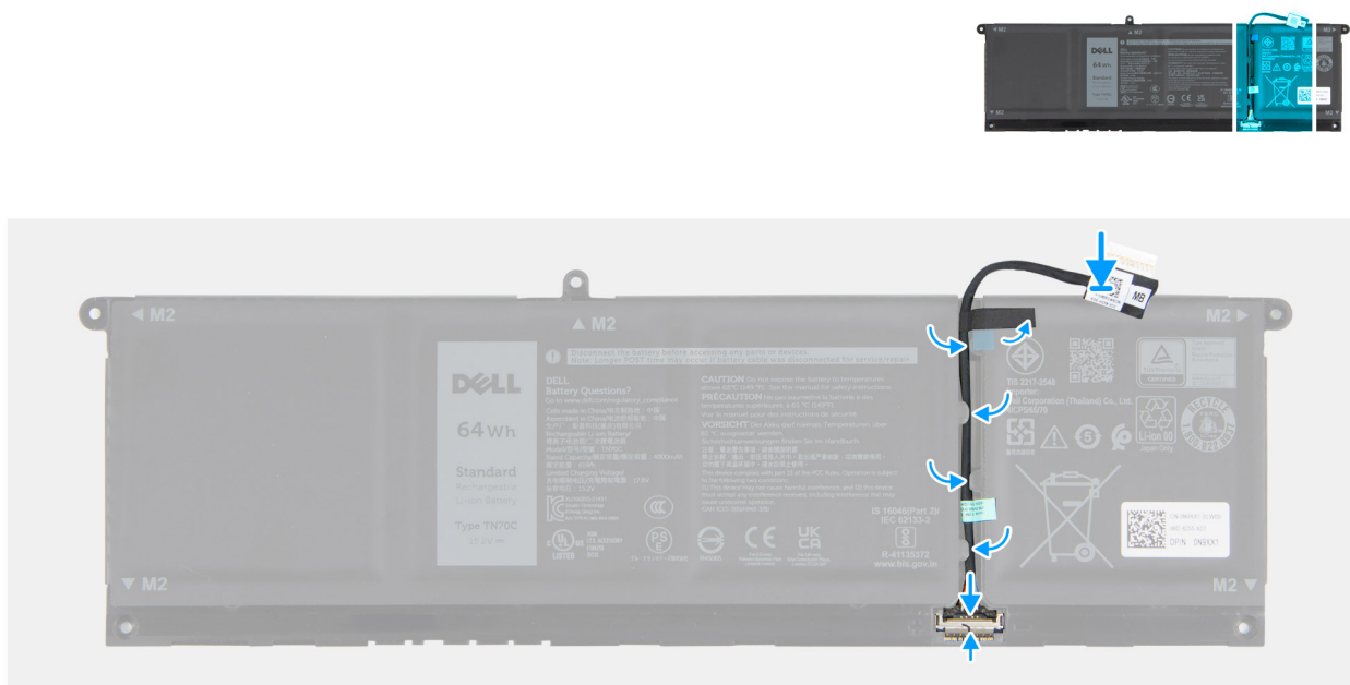
Figure 21. Connecting the battery cable
