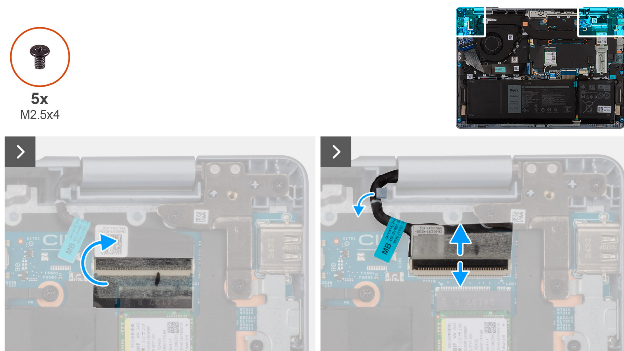
Figure 42. Disconnecting the display cable
