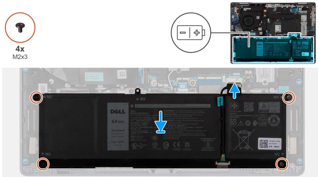
Figure 19. Installing the battery
